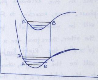
Thus a plot of intensities of the bands of a system in a (v'-v") among and join up the most intense bands, we obtain a parabolic curve. It is called the "Condon Parabola"
